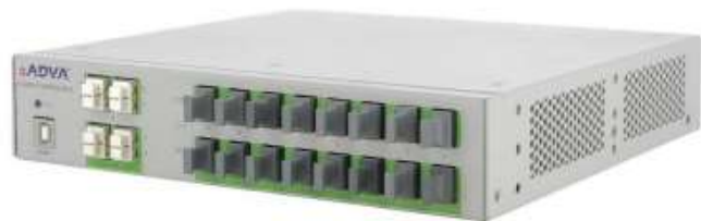
MPO based port extender 16 x MPO24 = 384 ports
